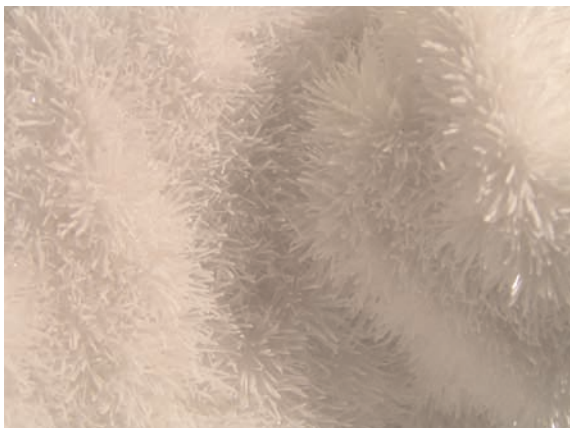
NEAT Gotthard: Laumontite needles (about 10 mm long) cover a fissure wall in granite
